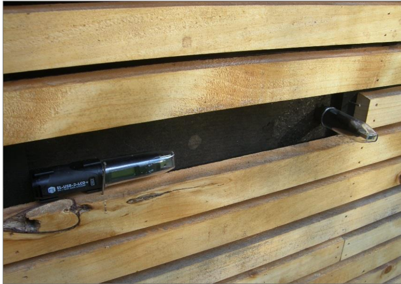
Figure 6. External sensor placement, house
